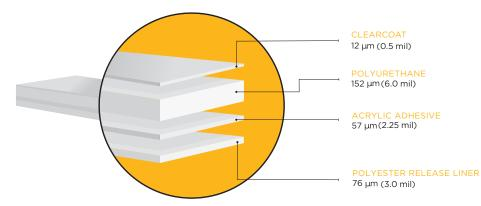
NOMINAL THICKNESS W/O RELEASE LINEF 221 µm (8.75 mil) +/- 10%
